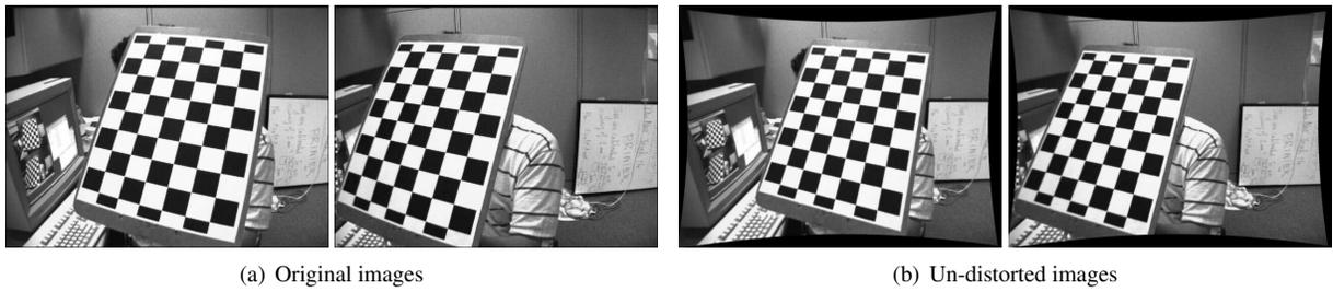
**Fig. 3.** Example of stereo image un-distortion with a planar target.
