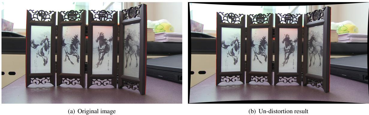
**Fig. 4.** Example of un-distortion by “transferring” un-distortion parameters to a new image sequence. Two red vertical fiducial lines are added to the image to illustrate the distortion (a) and un-distortion effect (b).
